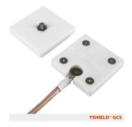
YSHIELD GmbH & Co. KG Rotthofer Straße 1 94099 Ruhstorf, Germany Further information: www.yshield.com, info@yshield.com Grounding connection with two plates that get screwed together. For all electrically conductive fabrics, fleeces, meshes. The two connecting plates must be screwed together - the material that is supposed to be grounded needs therefore to be perforated.
